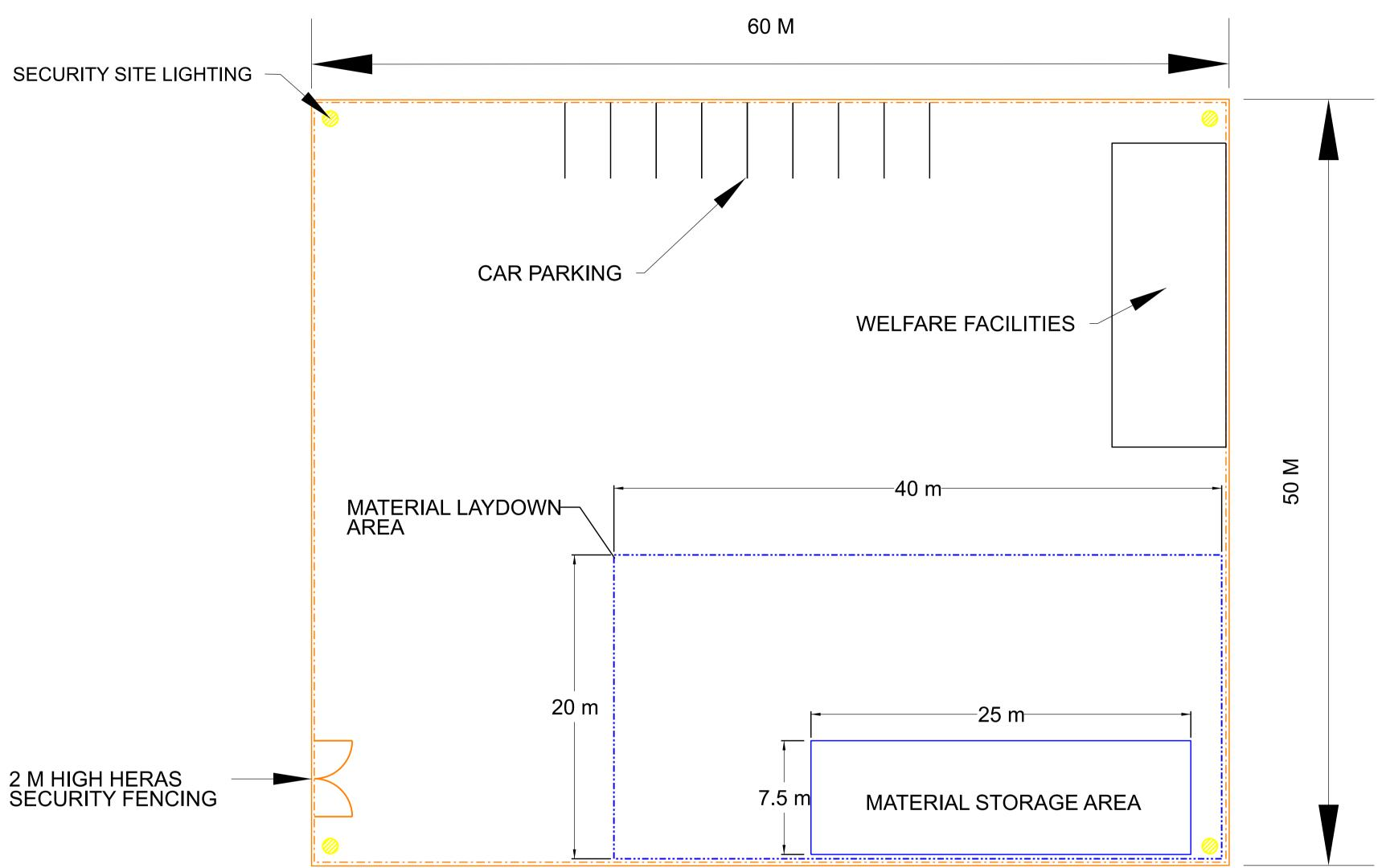
TEMPORARY CONSTRUCTION COMPOUND/ LAYDOWN AREA SCALE 1:200
